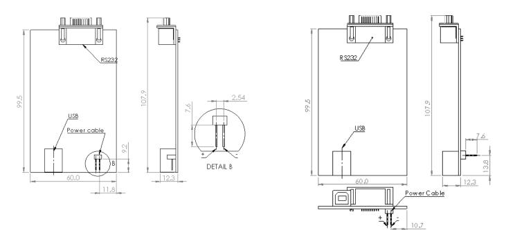
**Note:** The DC Power Barrel Jack Connector can be replaced with a two-pin connector, available in two configurations: one with pins facing downward for direct PCB mounting and another for connection with a standard cable connector. This flexibility allows for integration into various system designs.
