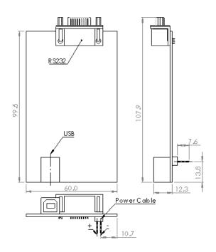
**Note:** The DC Power Barrel Jack Connector can be replaced with a two-pin connector, available in two configurations: one with pins facing downward for direct PCB mounting and another for connection with a standard cable connector. This flexibility allows for integration into various system designs.
