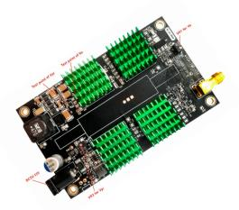
This NP series of fast-speed driver is designed to control the Premium NS series of solid state variable optic attenuators (VOA). The push-pull output design is especially suitable for driving capacitive VOA loads, assuring the fast response time both on rising and falling of attenuation. The VOA attenuation is controlled by 0-5V signal input. A wall plug power supply is provided for each driver.
